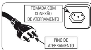
FIGURA 8.1 - CONEXÃO DO PLUGUE A TOMADA (MONOFÁSICO)
